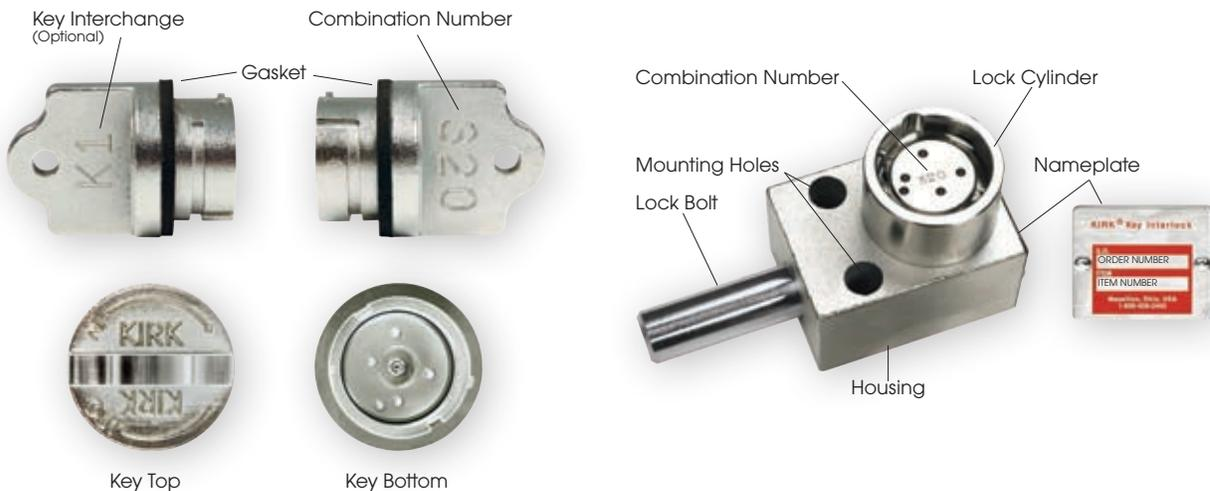
The KIRK MD Series and HD Series interlocks employ an oversized key that is designed to be extremely tough. The precision drivers located on the inner key disc are not susceptible to wear and slippage like etched style keys. The sealing gasket on the key, when used with the optional cover, prevent debris from entering the cylinder of the interlock.
