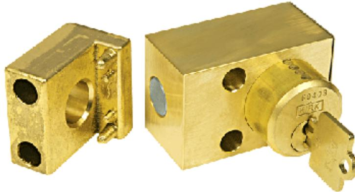
A Type D interlock has two parts: a main body with one or more cylinders and a latch block. The main body is typically attached to a door or hatch that swings open. The latch block is typically bolted to the door frame.
