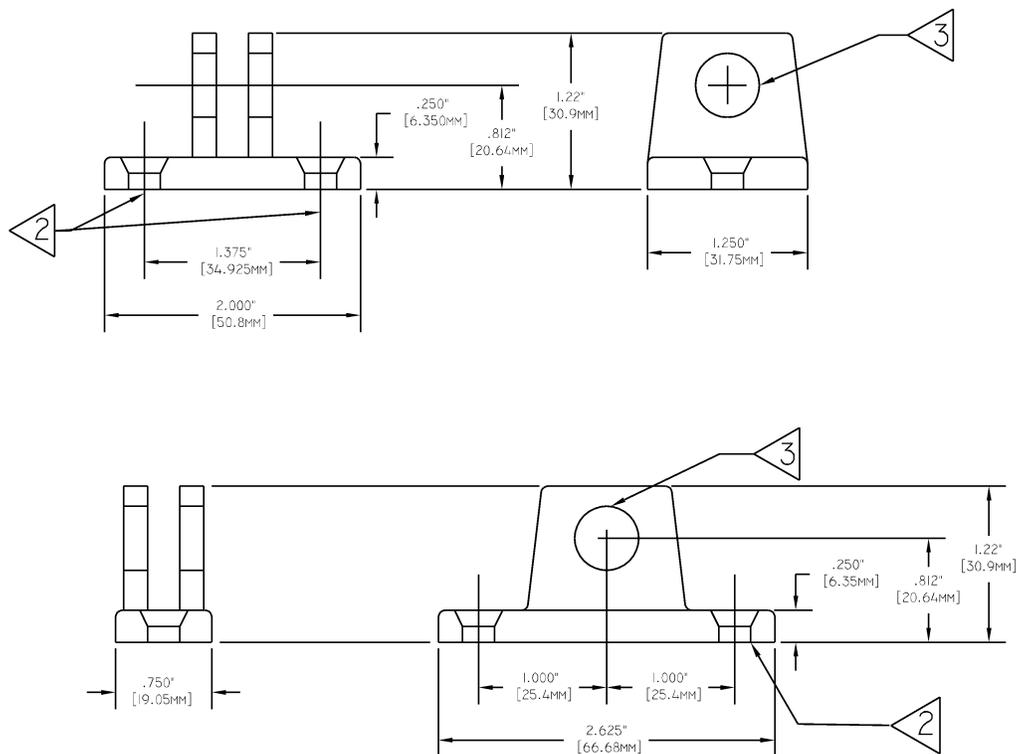
LONGITUDINAL Latch Block-Eye Bolt shown at top.
