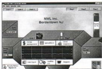
Total-view, total control —with PCAMS/NT's graphic-user interface which provides an at-a-glance summary of all critical ESP operating parameters.
